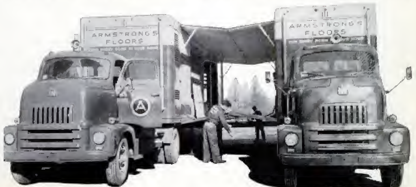
By parking two big trucks, each with expanding walls, alongside each other and coupling them as shown below, this company hauls its own mobile auditorium seating 100 persons anywhere in the country for sales meetings
